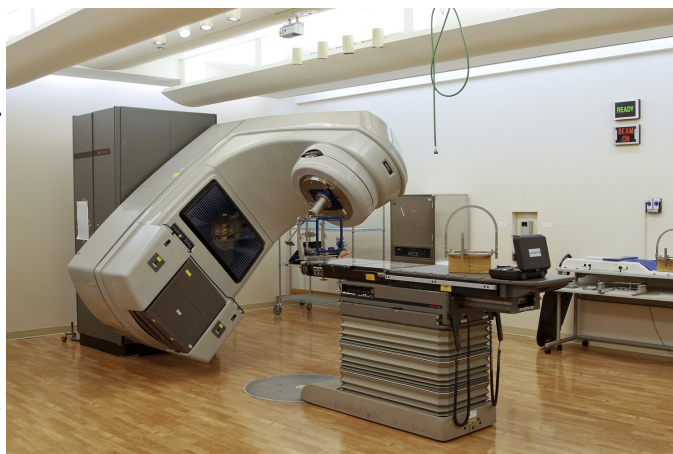
Linear accelerator, one of the high technology machines used to deliver radiation therapy. (Photo source: National Cancer Institute. Creator: Daniel Sone.)
